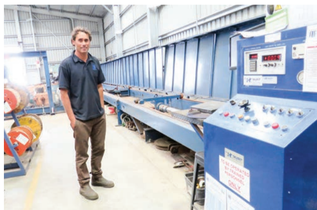
LEFT: Ben with the 100 tonne test bed which measures the tensile strength of lifting equipment. ABOVE: A Talurit hydraulic crimper
