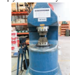
LEFT: Ben with the 100 tonne test bed which measures the tensile strength of lifting equipment. ABOVE: A Talurit hydraulic crimper
